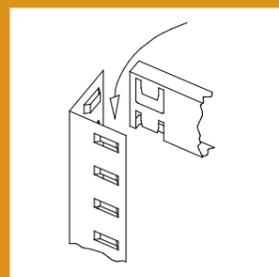
Assembly of snap-fit racks
