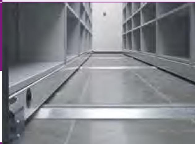
The trackage is galvanized. The total height of the track is 12 mm. Trackage is anchored to the floor with expansion bolts. The outermost tracks have an anti-tilt system, protecting against overturning. Optimally selected number of rails ensures smooth and easy movement of units. There is also a possibility of installing a chain in the trackway.
